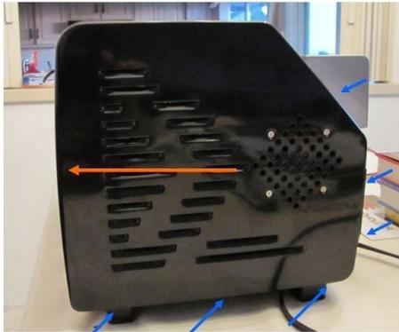
Remove 6 screws (blue arrows), slide panel forward (orange arrow) set panel aside
